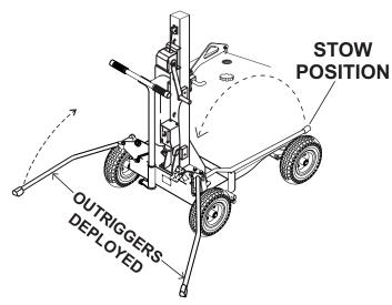
Figure 9. Outriggers (Deployed Position)
